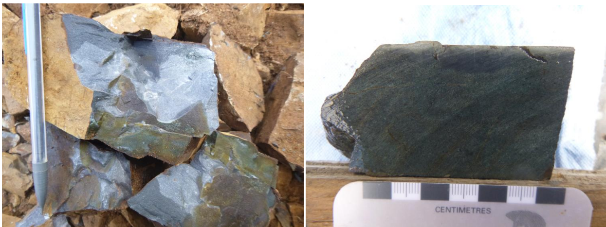
Figure 5. Photoplate hornfelsed sedimentary rocks. Left and right: Fine grained hornfelsed siltstone, locally 1 to 3% py +/- po, locally with biotite.
