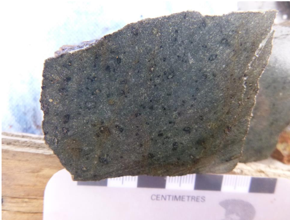
Figure 7. Photo of hornfelsed volcanic rock. Hornfelsed volcanic with lithic fragments and amphibole +/- feldspar crystals.
