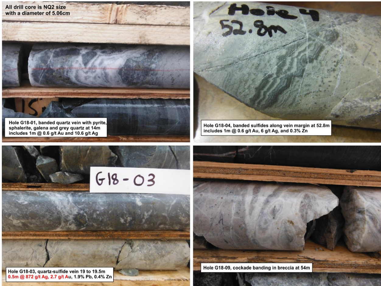
Figure 10. Photographs of select vein textures within and around mineralized zones from 2018 drilling. Hole number and depth are indicated on each photo.
