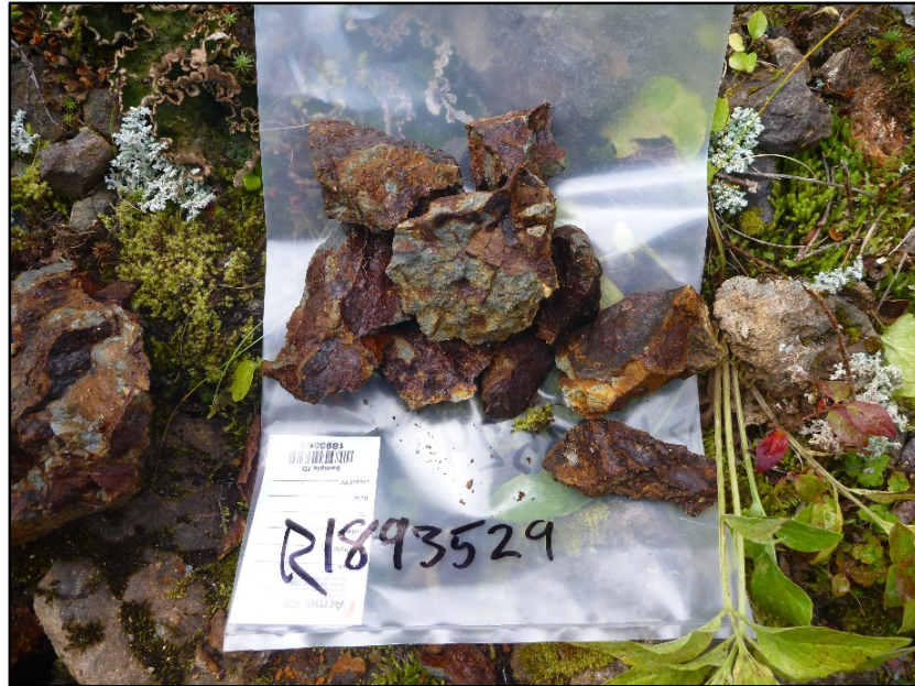
Figure 8: Sample R1893529, fractured and pyritic mafic flow volcanics
