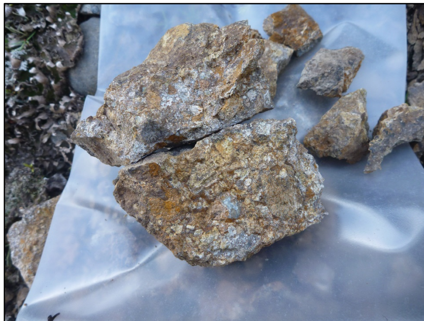
Figure 9: Sample R893535, brecciated mafic volcanics
