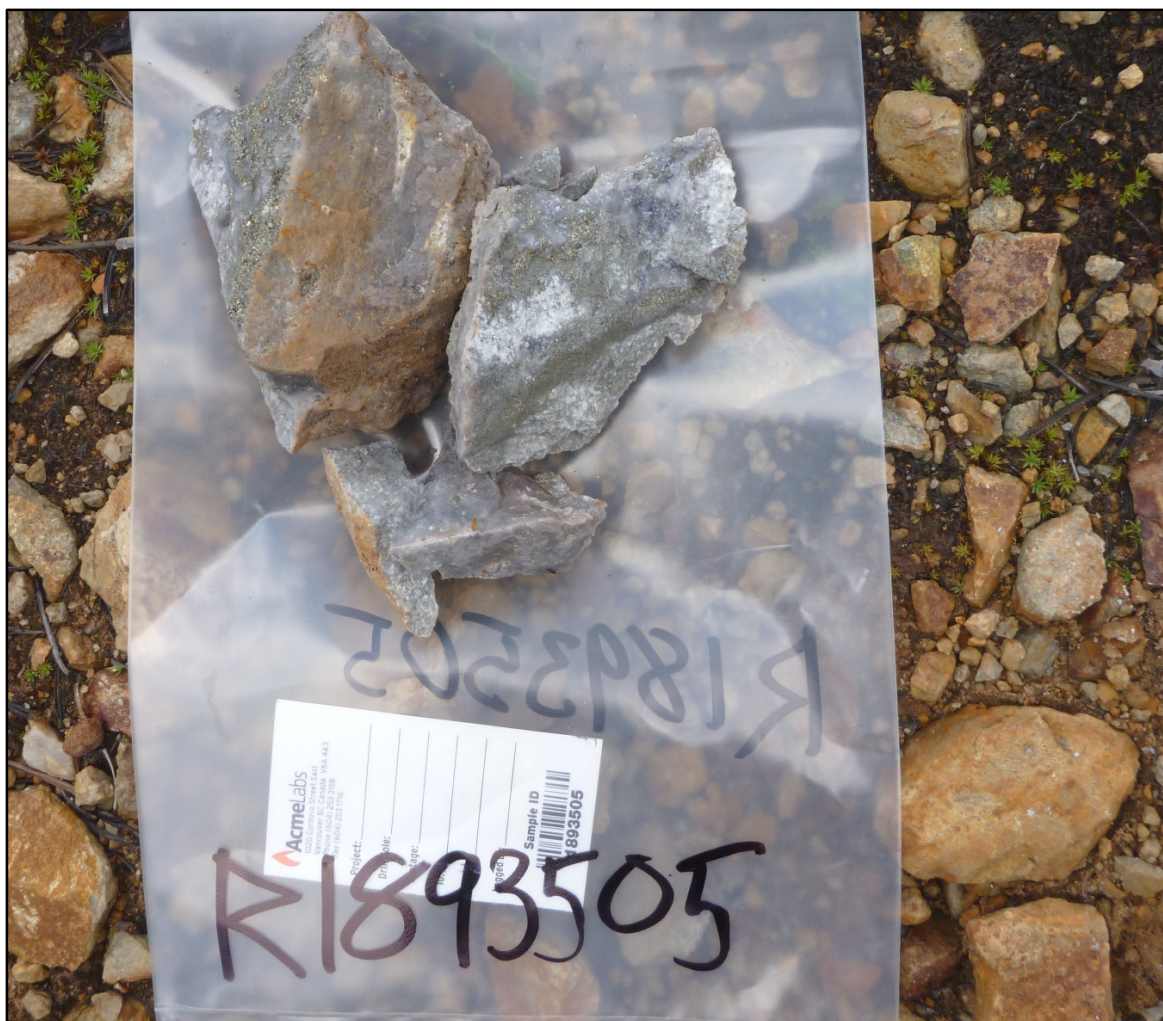
Figure 14: Sample #1893505, Quartz-Molybdenum veining, central deposit area
