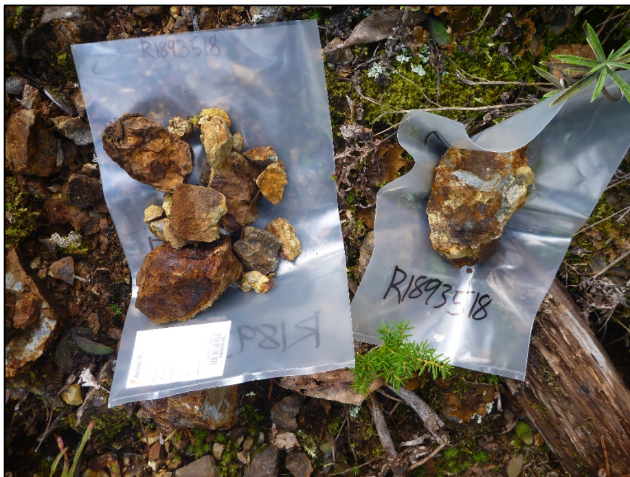
Figure 7: Sample R1893518, Pyritic conglomerate near terminus of drivable road
