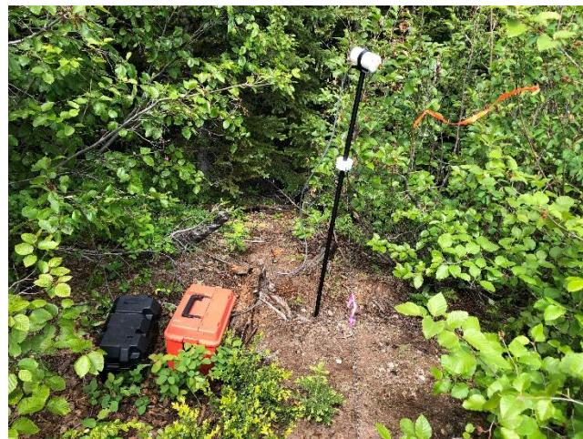
**Figure 4 – Magnetic Base Station at Nicoamen Property, June 8<sup>th</sup> 2019**
