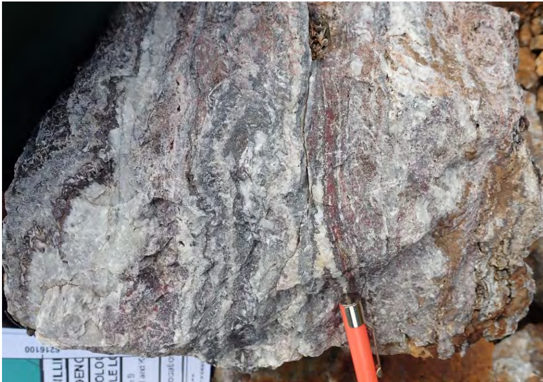
Plate 6: Quartz-barite-hematite-magnetite-sulphide vein, Independence Showing. From Trench/Pit 5
