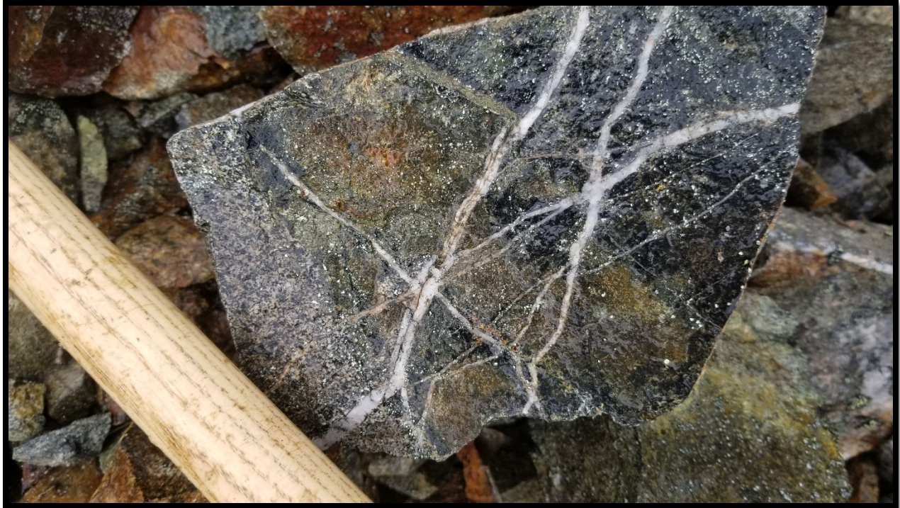
Figure 7-1. Monzodiorite (left) cutting diorite (right) with stockwork of quartz-K-feldspar veins which cut earlier epidote-pyrite veins (on surface) and several K-feldspar veinlets within the monzodiorite on the left side of the rock.
