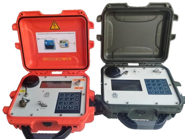
**Figure 2-3: Single Channel Current Recorder and dual Channel Voltage Receiver (Alphi).**
