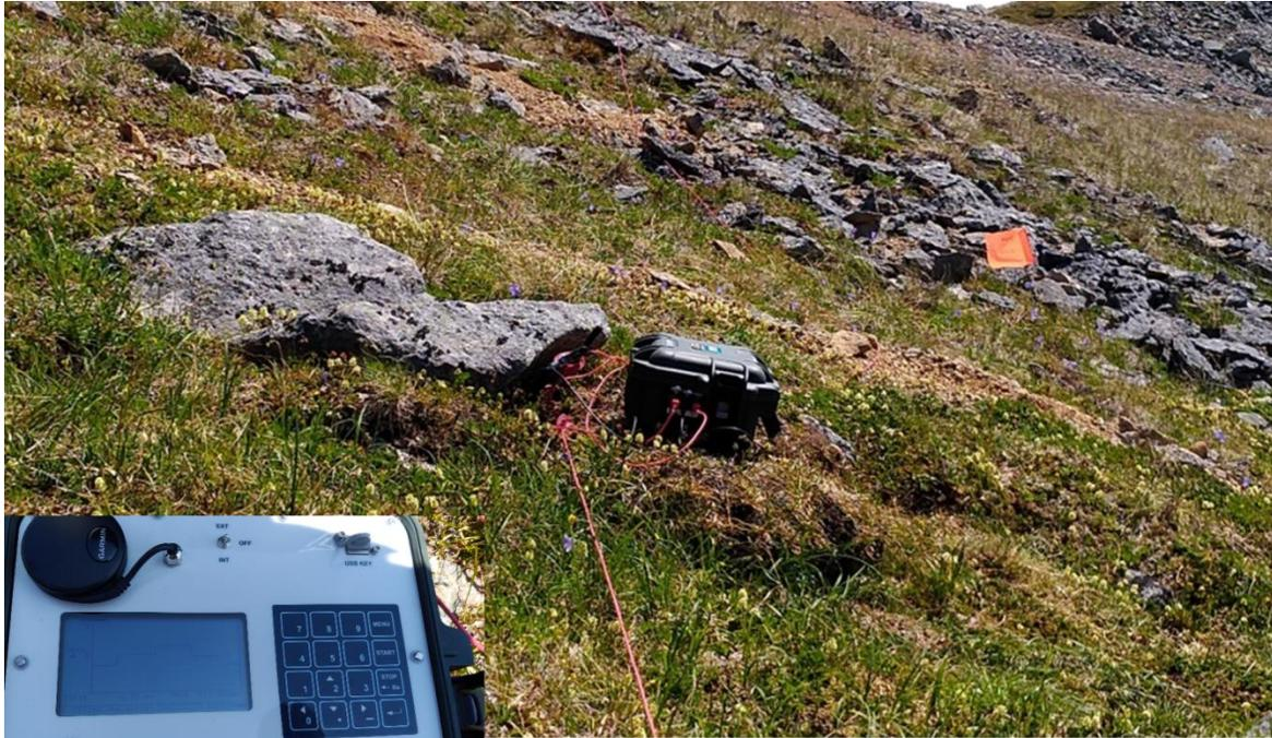
**Figure 2-6: Field setup of wireless IP receiver (Alphi), orange flag marks the location. Inset screen image shows full waveform signals.**
