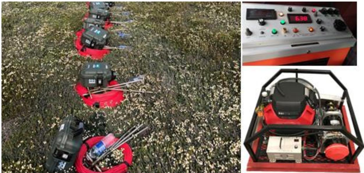
**Figure 2-7: Alphi with dipole wires and stainless steel electrodes, Honda Motor Generator MG 12A, 10 KW Transmitter used in the field.**
