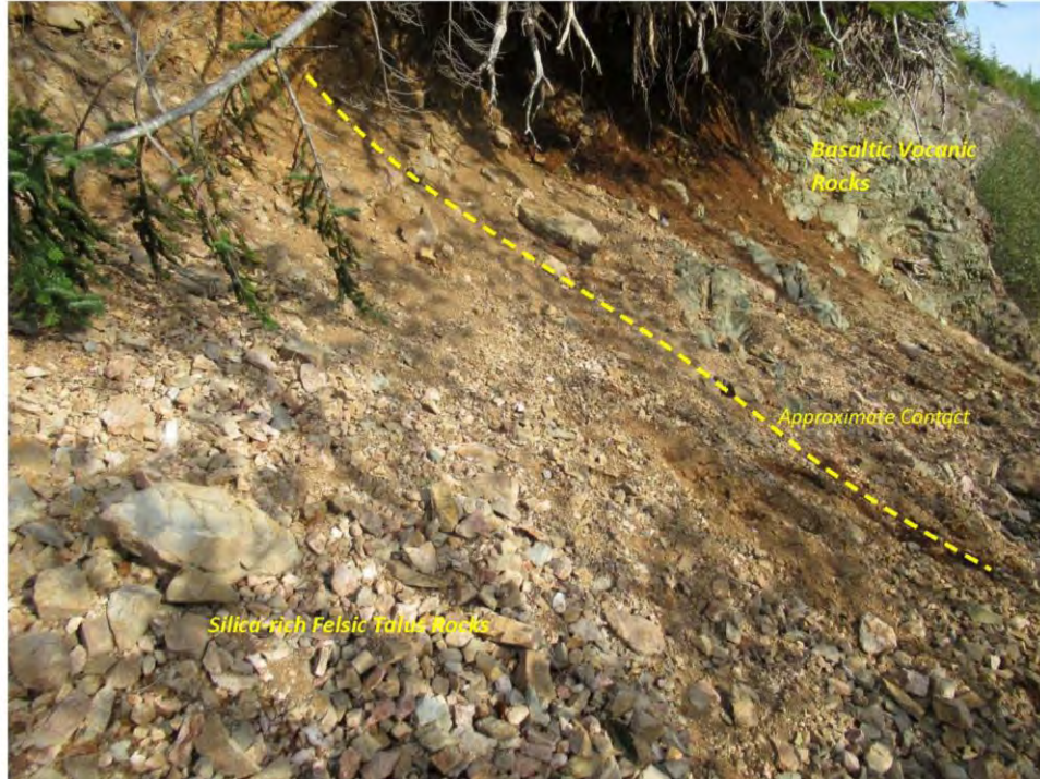
Photo 3 shows northeastern section of road cut showing basaltic volcanic rock outcrop in approximate contact with silica-rich talus. Dominant talus material consists of thinly laminated silica-potassic layering.
