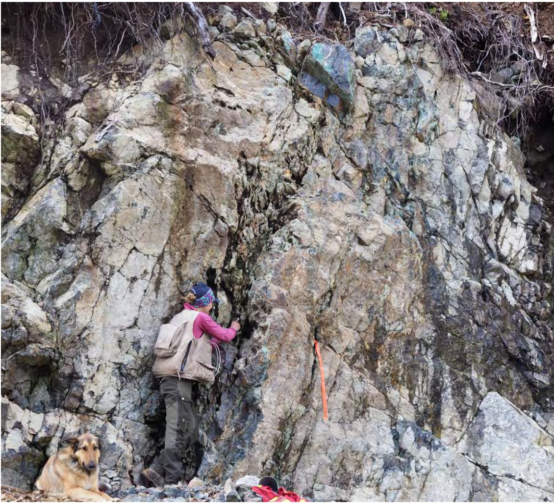
Plate 8: 1 m Wide Bornite-rich Shear Zone, Sisters Copper Showing
