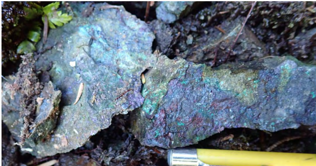
Plate 4: Bornite-chalcopyrite-rich Vein, Boyes Creek
