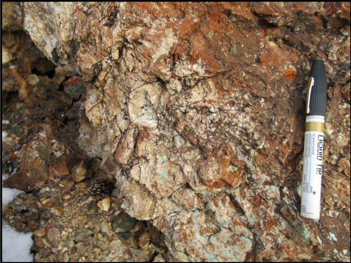
Photo 7: Close-up view of a typical mineralized, iron carbonate (dolomitic) breccia containing kaolinite-quartz-calcite and limonite fragments with occasional, smaller cryptocrystalline agate-like fragments.
