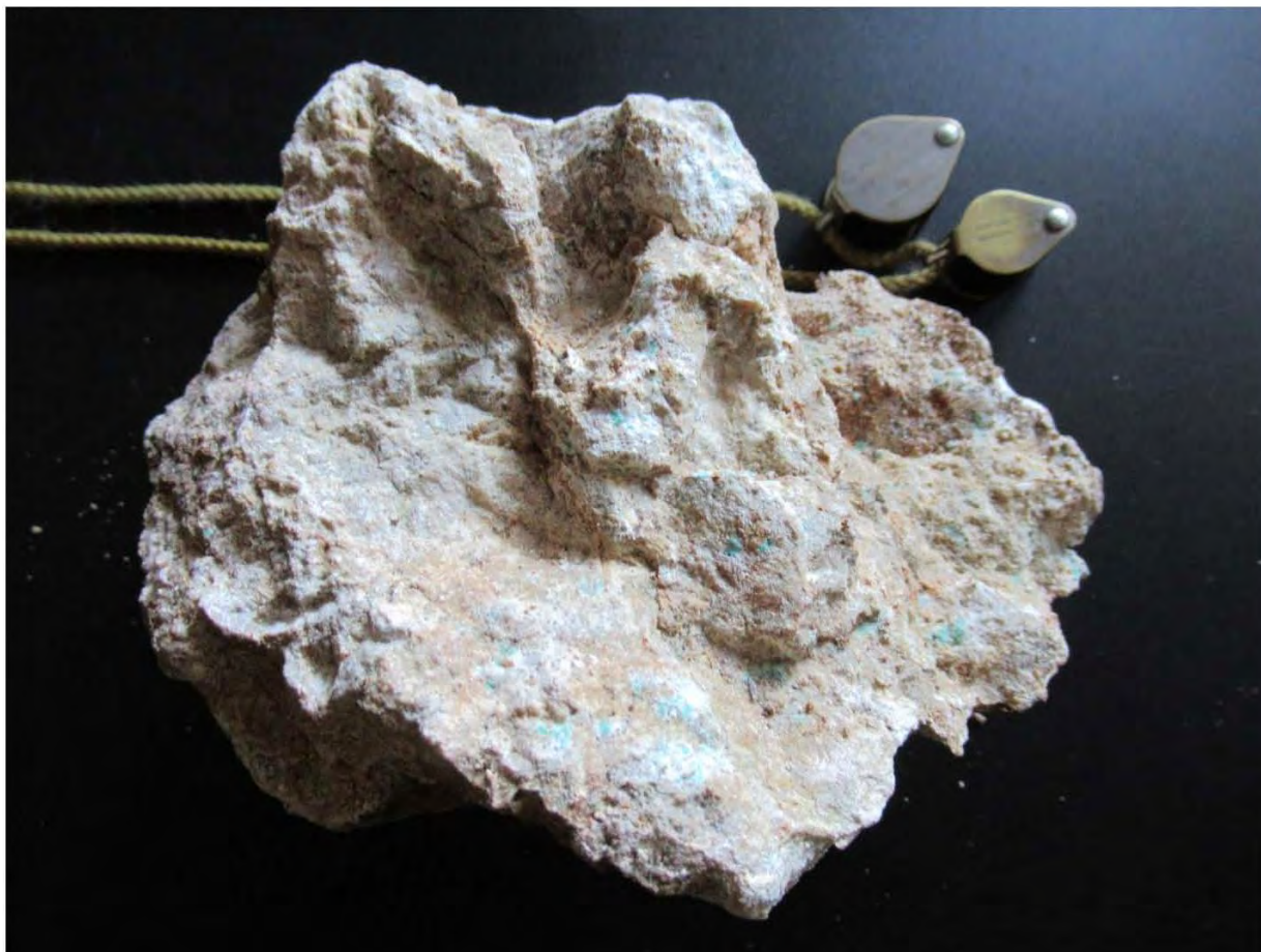
Photo 8: Sample collected adjacent to the adit entrance displaying intense iron carbonate-kaolinite altered breccia carrying malachite fragments.
