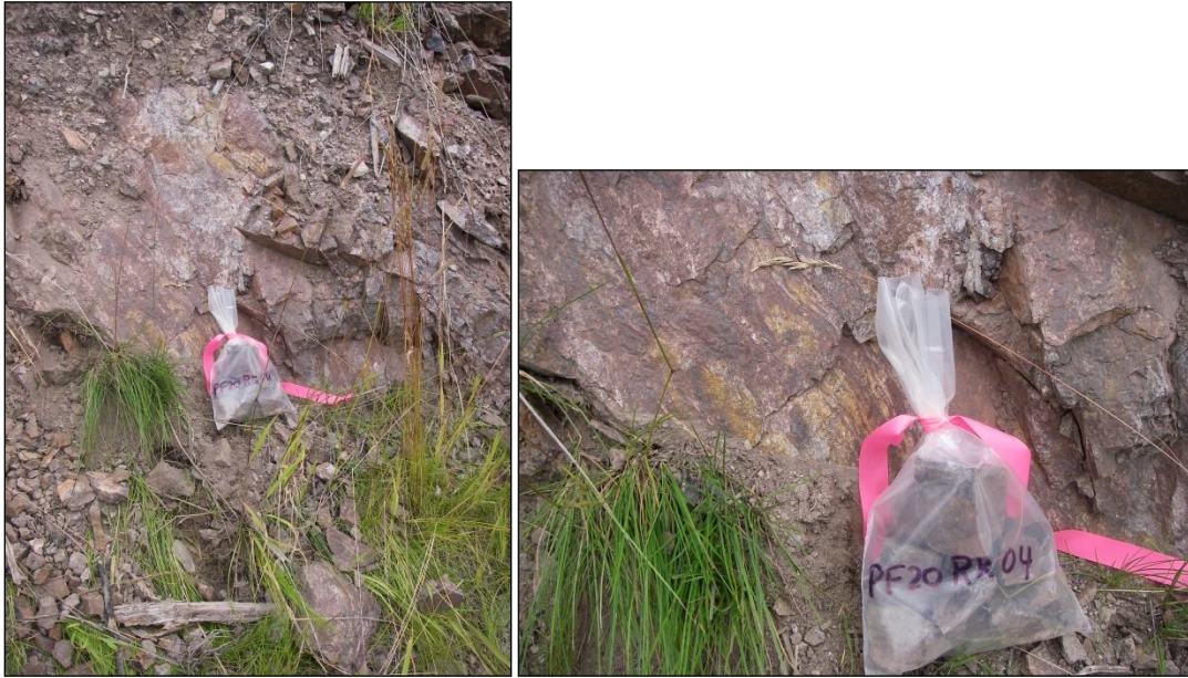
Figure 19 Proof Rock Grab PF20RK04 Sample location (left) and sample (right) volcanic rock with oriented quartz-sericite(?) flow patterns and pervasive hematite.
