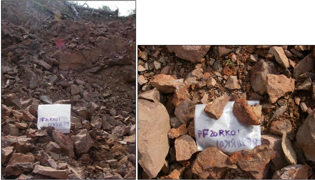
Figure 17 Proof Rock Grab Sample PF20RK01 location (left) and sample (right) – fault gouge striations evident with bladed white quartz crystal and pervasive hematite.
