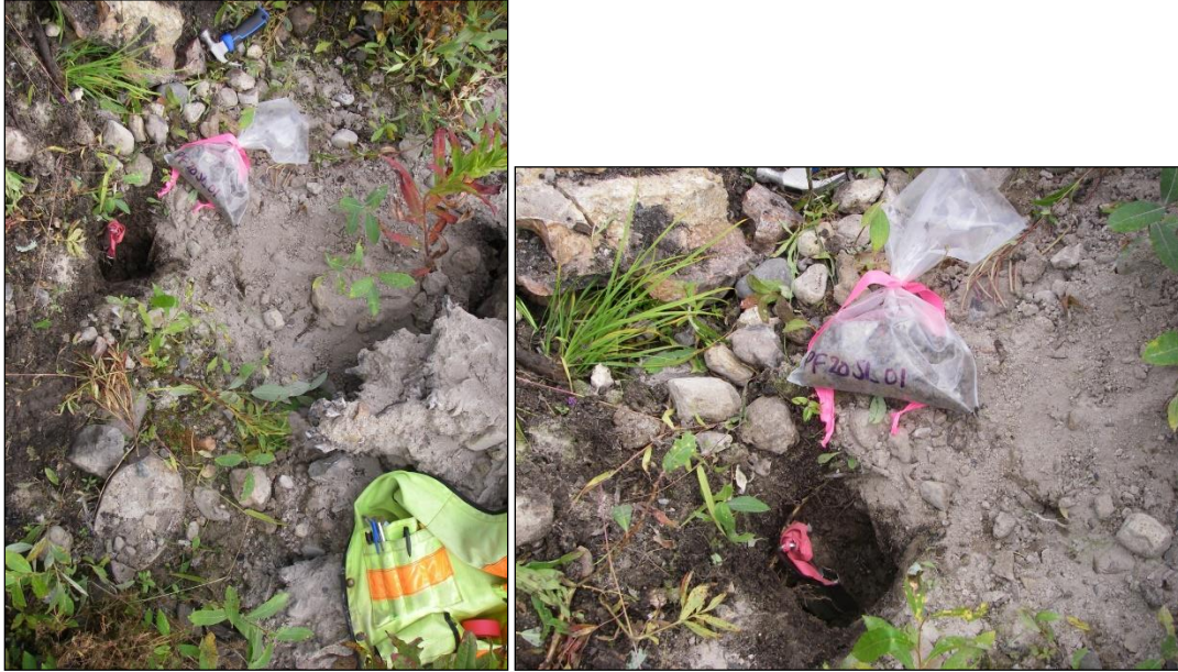
Figure 21 Proof Soil PF20SL01 Sample location (left) and sample (right) collected from under an overturned tree stump in old cut block approximately 40 cm beneath the duff and 20 cm from current surface (~ 60 cm deep).
