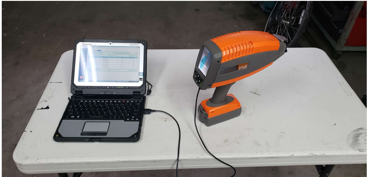
Figure 1. The handheld Terraspec Halo SWIR ASD device.
