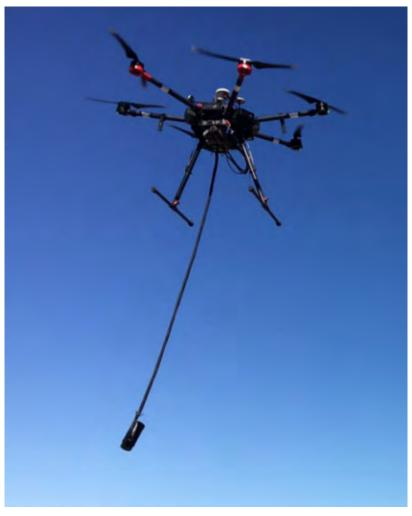
Figure 5: UAV Magnetometer System Configuration
