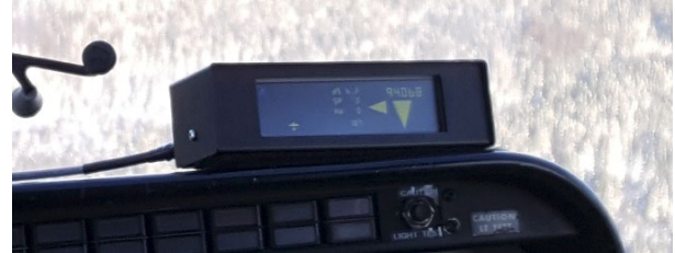
Figure 6 – Pilot Steering Indicator and Radio Altimeter Indicator
