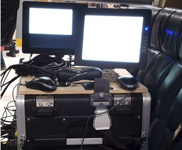
Figure 5 – EGL Navigation Computer, Moving-map Display
