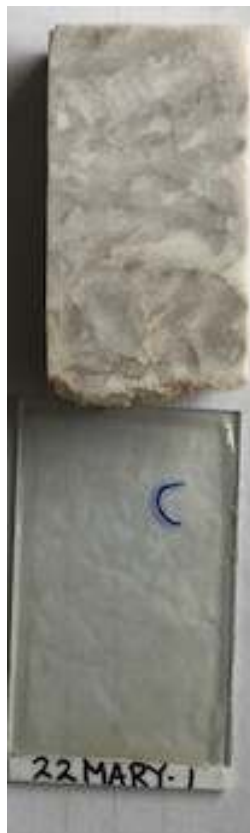
Overview of thin section and offcut (blue semi-circle marks photomicrograph location).
