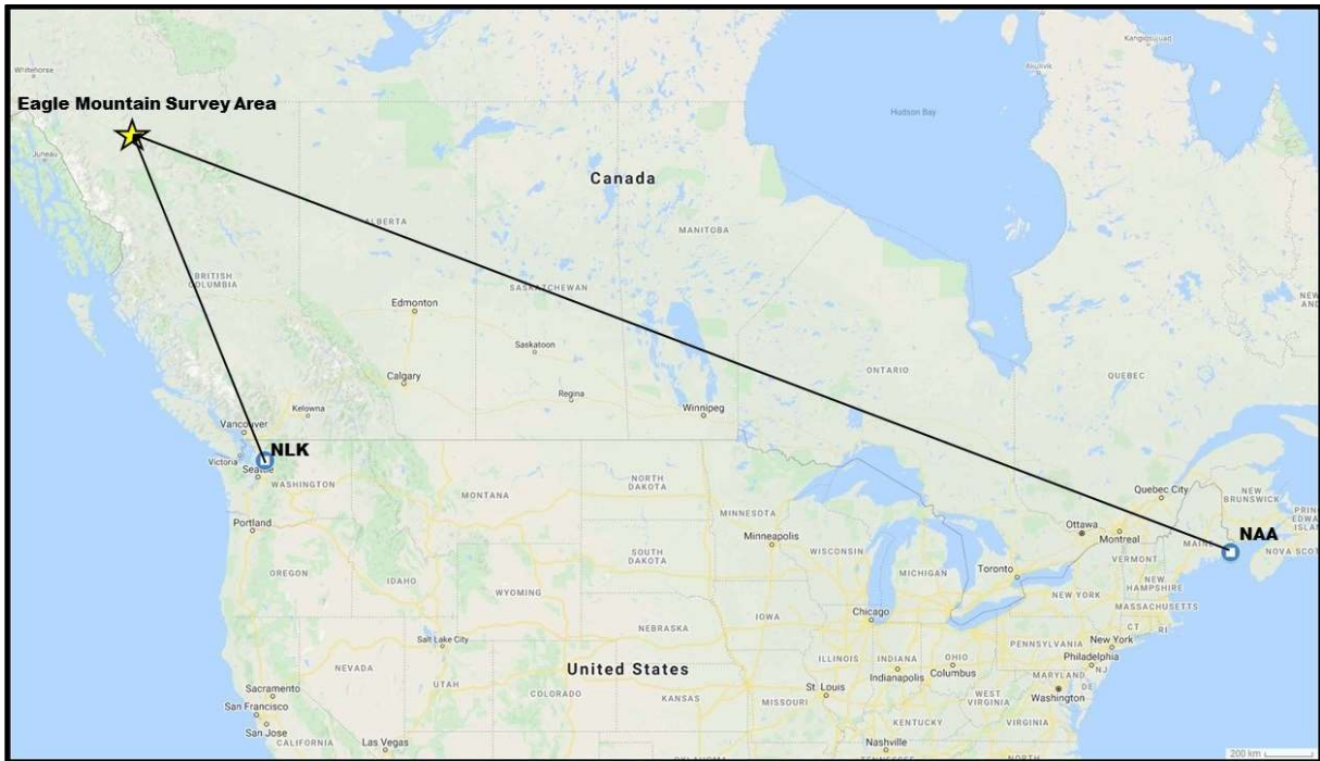
Figure 20: NLK and NAA VLF transmitter stations relative to Eagle Mountain survey block.
