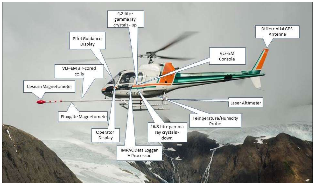
Figure 6: Survey helicopter equipped with a magnetic sensor for magnetic data acquisition, VLF-EM system, and gamma spectrometer.
