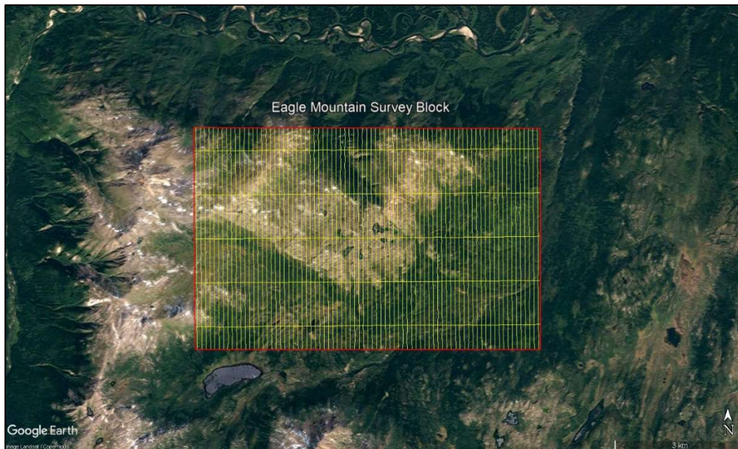
Figure 3: Plan View – Eagle Mountain survey block with actual flight lines in yellow, survey block boundary in red.
