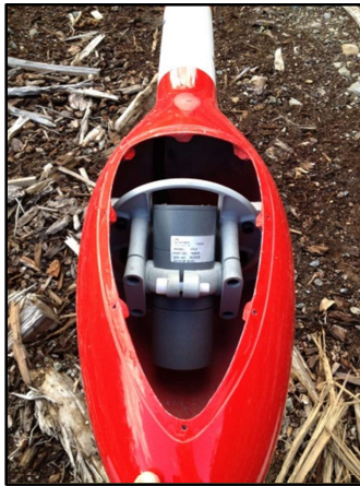
Figure 13: View of "stinger" configuration with magnetic sensor.
