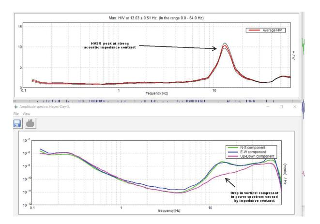
From processing the data we know the peak resonant frequency but there are still two unknowns. Vs and the thickness (h). In order to accurately calculate the thickness for each location, we need to know the shear wave velocity of the overburden layers. That can be acquired by running a test station at an area of known depth such as a drill hole. Once the velocity is known it is simple to calculate the thickness.
