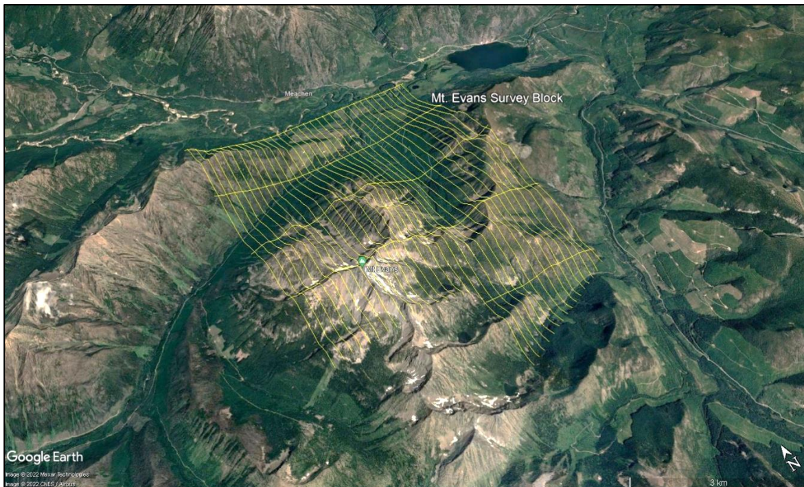
Figure 4: Terrain View – Mt. Evans survey block with actual flight lines in yellow.
