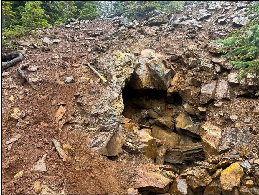
Plate 1: unnamed adit. The entrance has collapsed and the location is not noted in historical reports but a large red waste dump makes it easy to locate from the air. The workings appear to have exploited mineralized quartz veins at the contact between a gabbroic intrusion and metamorphosed sediments of the middle Aldridge Formation.
