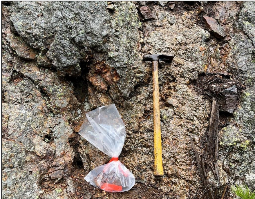
Plate 3: Sample KBAKR003 collected from a 1.0-1.5m wide shear brecciated hosted within a gabbroic intrusion. The Blue Peter adit appears to be exploiting mineralization that forms along the intrusive margin. Clast composition includes angular gabbro and quartz vein material.
