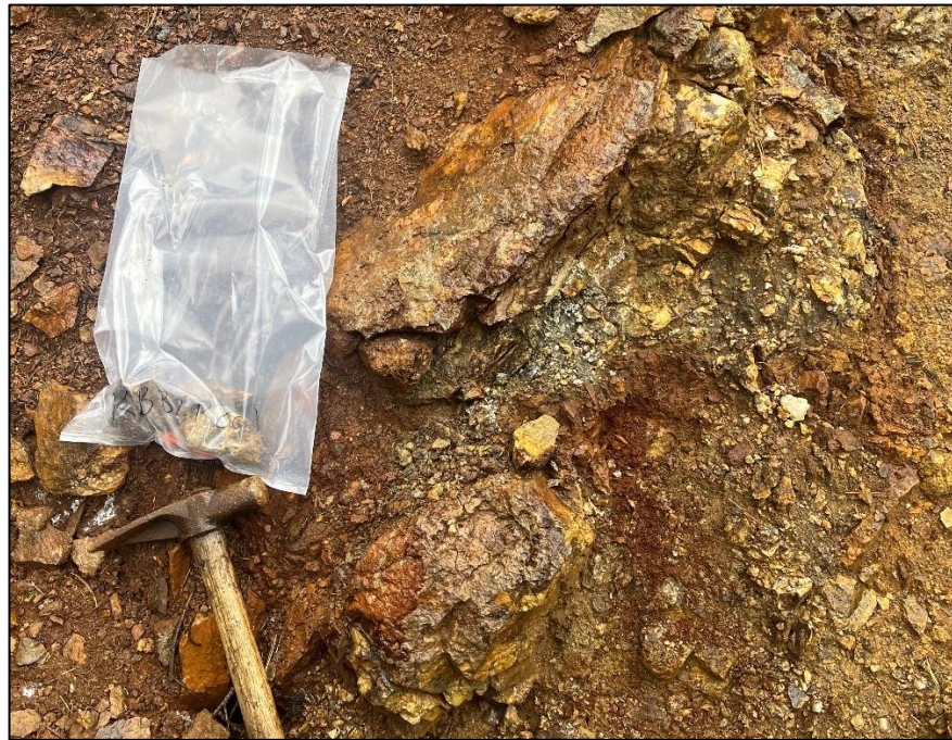
Plate 2: Sample KBAKR001 contains mineralized quartz veins up to 5 cm wide. The sample returned 1.24 g/t Au.
