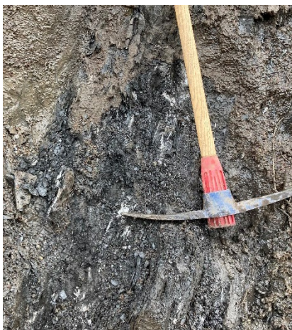
Figure 7 Shaly Material w/ laminations near Area 2
