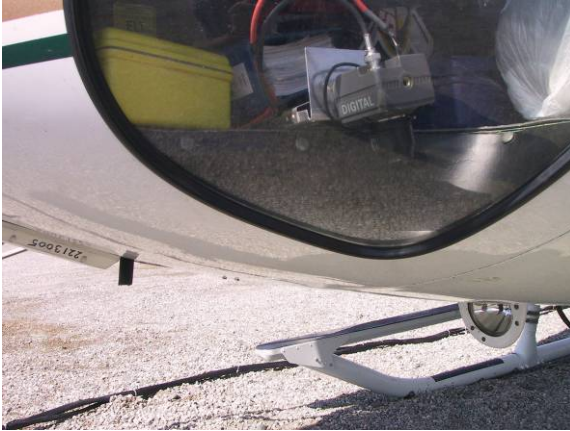
Figure 9. Digital video camera typical mounting location.
