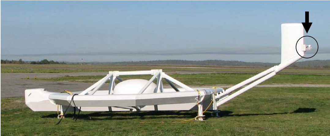
Figure 4. AeroTEM II EM bird. Arrow indicates the location of the second cesium magnetometer sensor.
